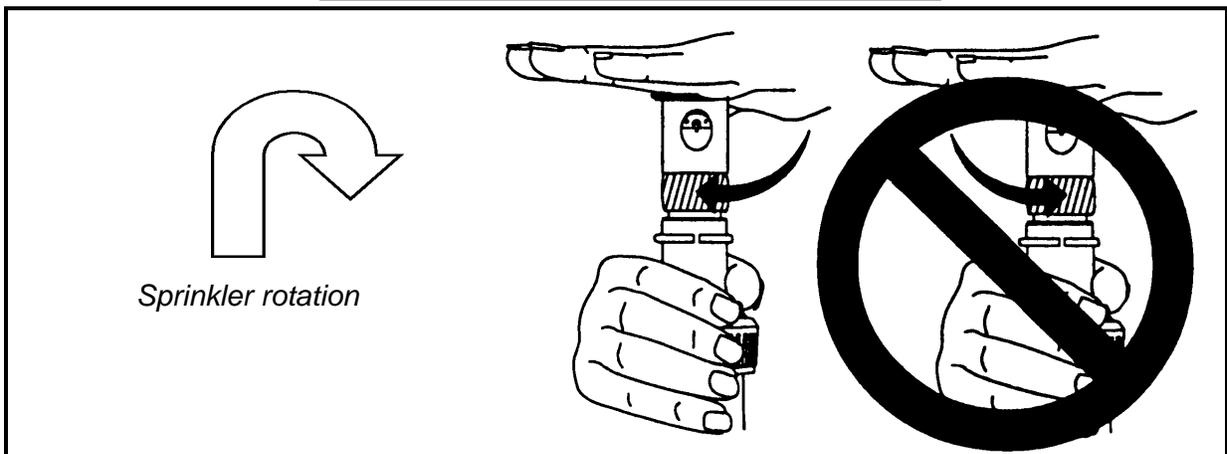
Always turn head in the same direction the sprinkler is rotating. Turning the head against the sprinkler's rotation may damage the sprinkler.
